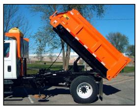
Each of our GI combination spreader/dump bodies is equipped standard with underbody hoist, polymer spinner with hydraulic drive, polymer chute, conveyor chain cover and hose guide kit (Guide kit available only for the GI-90T).
