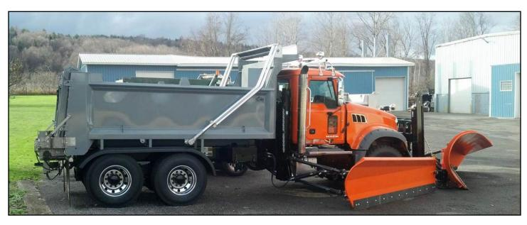
Everest MR Hi-tensile Dump Body Built with Hardox 450 material for optimum abrasion resistance and strength.
