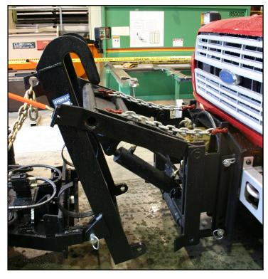
Driver has a work ready unit in mere seconds. Approach guides help the driver line up the male and female section during coupling.
