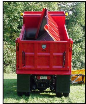
Spinner assembly is adjustable to allow you to spread material where you want it. With our adjustable metering door it allows you to limit or increase the amount of material that you move to the spinner. The hydraulically powered spinner disc is 18" round with six (6) vanes. The spinner assembly can be removed for summer use. The chute can be rotated 90° to spread material to the center of the road.
