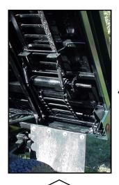
Conveyor uses 667X type pintle chain at 12" wide with 3/8" x 1-1/4" flites on 4-1/2" centers. The conveyor is self cleaning drag chain powered through a 10:1 reducing gearbox and hydraulic motor.
