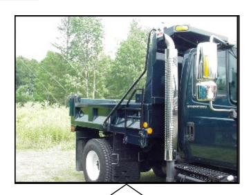
"SDSL" side dump spreader body can be used either as a salt and sand spreader application or as a conventional dump body. The dumping action is achieved by the use of a direct mounted 8" bore by 21" stroke double acting cylinder.
